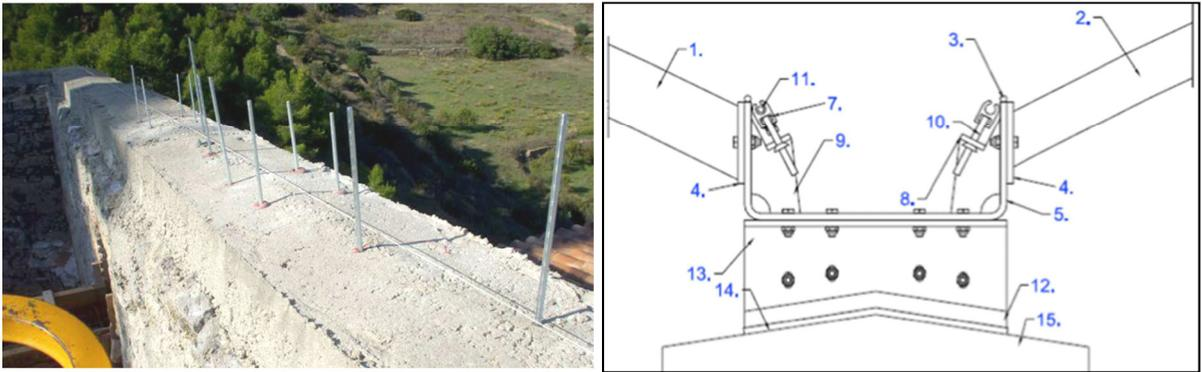
Fig.10: Reinforced concrete ring on top of the walls. Fig.11: 1 CHS 101.6x3.6; 2 CHS 76.1x3.25; 3 Ø10; 4 Cap; 5 Channel 400x180x6; 7 Keder rail; 8, 10: Tensioning system; 9, 12, 13 Gussets; 11 Polymer edge bead; 14,15 Ring.
