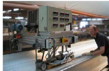
Figure 24, Principle of continuously working thermal impulse welding (release belt made of PTFE coated fabric)
