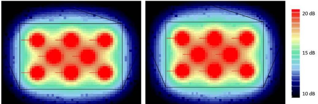
Figure 5: Sound strength  $G$ , as simulated from multiple sources equally distributed over the playground for roof shape 1, in height of 1.5 m (horizontal plane). Results at low frequencies (125 Hz) in case of ETFE (left) and glass roofing (right),
