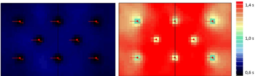
Figure 6: Reverberation time  $T_{30}$  (s) for cases with roof shape 2. Results at low frequencies (125 Hz) in case of ETFE (left) and glass roofing (right).
