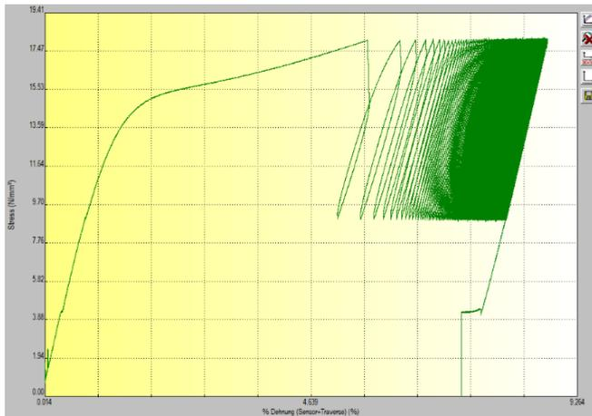
Figure 9: strain-stress diagram 250µm ETFE foil, 300 cycles; test for print stability
