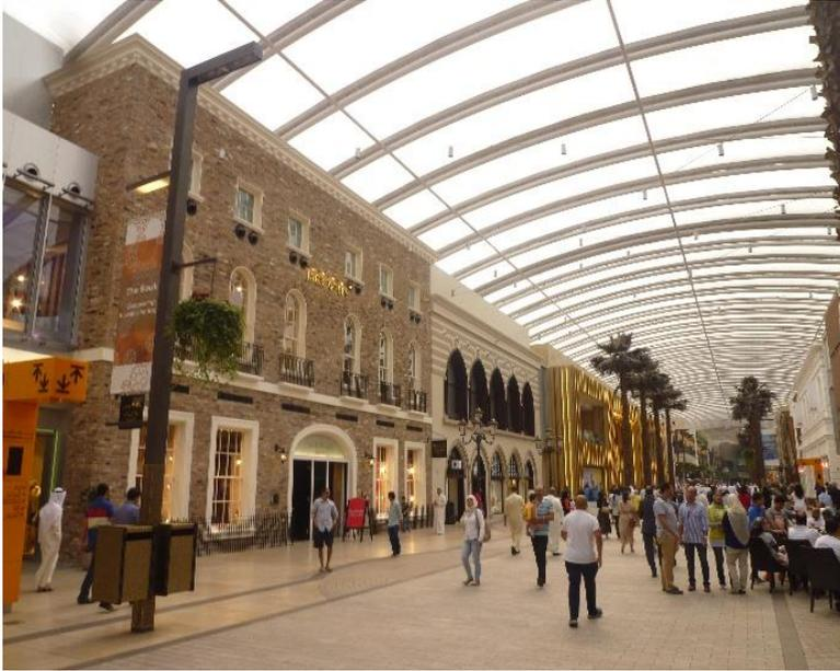
Figure 3 The Avenues Mall, Kuwait – Texlon® ETFE cladding system printed with DH 7:84 medium
