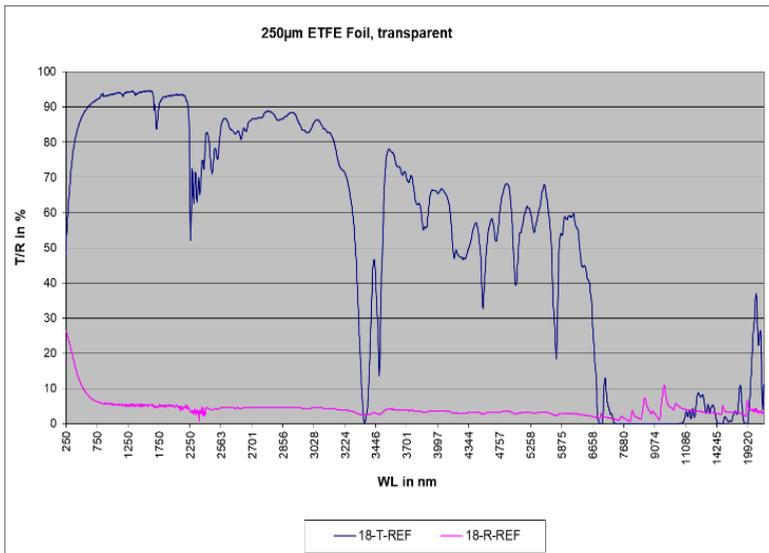
Figure 1: Transmission T and Reflection R of 250 µm ETFE foil up to 20.000 nm wavelength
