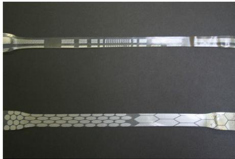
Figure 8: Two strips of ETFE after long-term corrosion test stressed with constant load of  $17 \text{ N/mm}^2$  at  $80^\circ \text{C}$  and 100 % humidity
