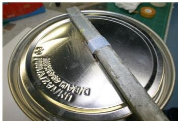
Figure 6: cap with small opening for ETFE stripe
