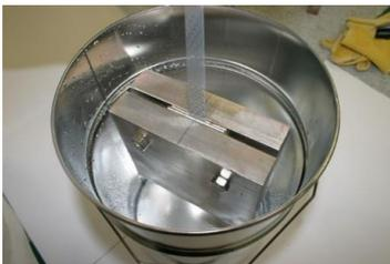
Figure 5: ETFE stripe loaded with weight up to 17 MPa
