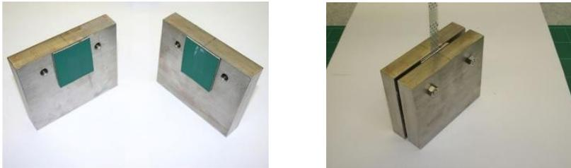
Figure 4: weight for creation of 17 N/mm<sup>2</sup> load on an ETFE stripe of 15 mm width
