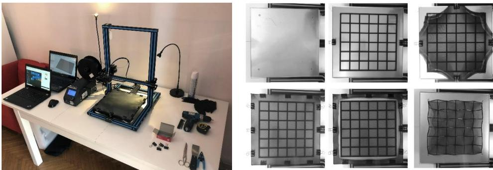
Figure 3: The Creality CR-10 3D-printer used by the team and six main steps of the fabrication process: (a) clean and pre-heat bed; (b) print lower layers; (c) stretch and clip fabric; (d) print upper layers; (e) cut away excess material; (f) remove part from printer bed and allow 3D deformation to occur.
