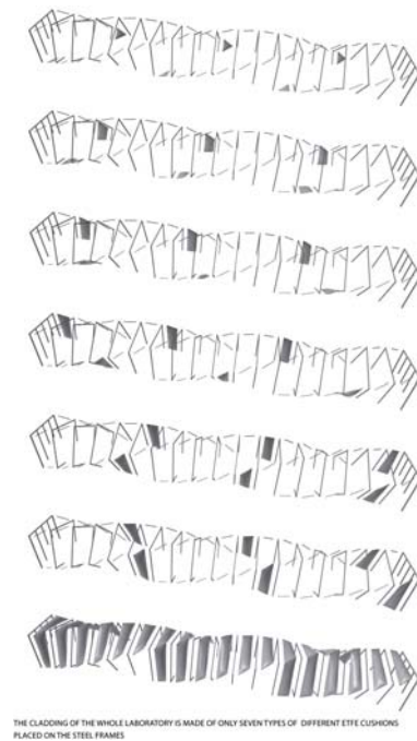
THE CLADDING OF THE WHOLE LABORATORY IS MADE OF ONLY SEVENTYPES OF DIFFERENT ETFE CUSHIONS PLACED ON THE STEEL FRAMES
