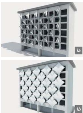
Figure 1. Conceptual visualisation of a kinetic facade system integrating a mechanically stressed membrane.
