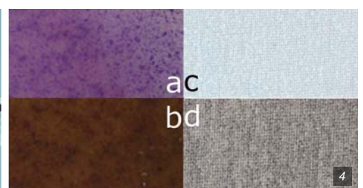
Fig. 4. Fabrics responsive to corrosive or toxic gases. Left: ammonia sensitive (a. no \text{NH}_3 ; b. in presence of \text{NH}_3 ). Right: hydrogen sulfide sensitive (c. no \text{H}_2\text{S} ; d. exposed to \text{H}_2\text{S} ). Samples are 1cm high.
