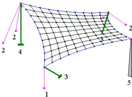
As we can see, only type 4 is what we would call traditional foundation. Type 3 could be considered traditional if the horizontal component was very small or if it was possible to establish a grid of straps between these and other footings. If not, we'll see that the design of the foundation is quite different.
