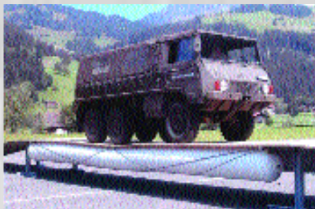
Figure 3. Temporary bridge spanning 8 m (First prototype)
