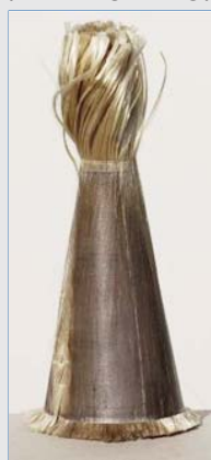
Fig. 3: The VECTRAN HT fiber cable with its termination moulded in a quasi-conical shape using an autogenous bonding technique
