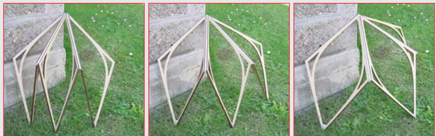
Fig. 19. Foldable model with textile junctions
