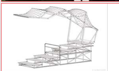
Fig. 9. Retractable Membrane Roof in the Courtyard of the City Hall in Vienna [Silja Tillner]
