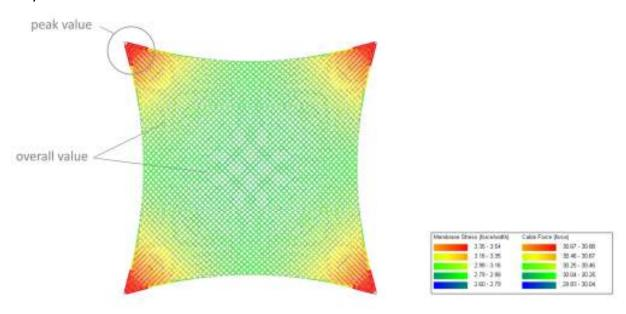
Figure 3: Representative drawing of the distribution of the stress in the membrane and the forces in the boundary cables
